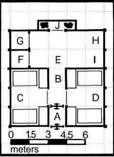
fresher (G) contains the toilet, a shower, and a basin for personal needs. Finally, the power plant (J) is a self contained power source for the entire structure, providing energy for the recycler, the galley, and for heat and cooling as necessary.
