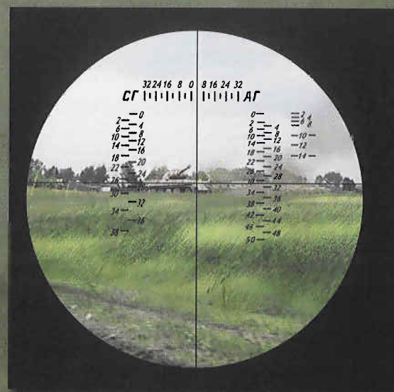
View through the TMFD-7 sight as an AP round ricochets off the Panther. Other than telling the driver to stop or the loader to load a shell there was little crew interaction.
