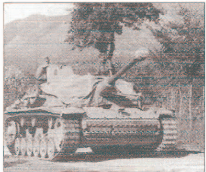
Long-barrelled StuG III of the Sturmgeschütz-Abteilung in Sicily, 1943. Judging by its 'untactical' appearance, with a tarpaulin blinding the fighting compartment periscopes and the external machine gun unmounted, this photo was taken before the Allied landings. (Robert Noss)
