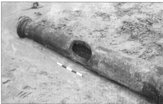
This bronze 'saker' ( sacre ) of Italian origin was recovered from the Spanish Armada vessel Juliana , wrecked off Streedagh Strand on the west coast of Ireland. It was subjected to an accident which blew out a section of the gun, demonstrating that some of the Armada weaponry was of dubious quality. (Dr. Colin Martin)
