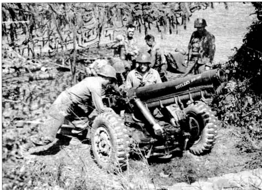
As German defenses in Brest stiffened the surrounding US forces brought in more artillery to lay siege to the port. This is an M3 105mm howitzer of the 9th Cannon Company, 2nd Division nicknamed "Hitler's Doom" preparing to fire on 28 August 1944. This lightweight howitzer was used in place of the heavier and more common M1 105mm howitzer in some infantry divisions in Normandy. Its maximum range of only 8,300 yards and lightweight construction limited its wider use.
