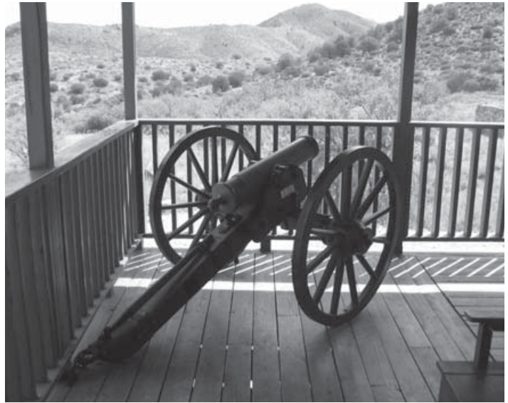
A muzzle-loading Hotchkiss 120mm mountain howitzer, photographed at Fort Bowie. This Napoleonic-looking little cannon, essentially unchanged since the French original appeared in 1827, was light enough to be disassembled and carried into rough terrain in pack-mule loads. Two of these were the decisive factor in the Battle of Apache Pass in July 1862. (Author's photo)
